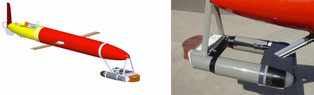
**Figure 3.5:** Zooglider schematic (left) and photograph of the Zoocam camera system (right)
