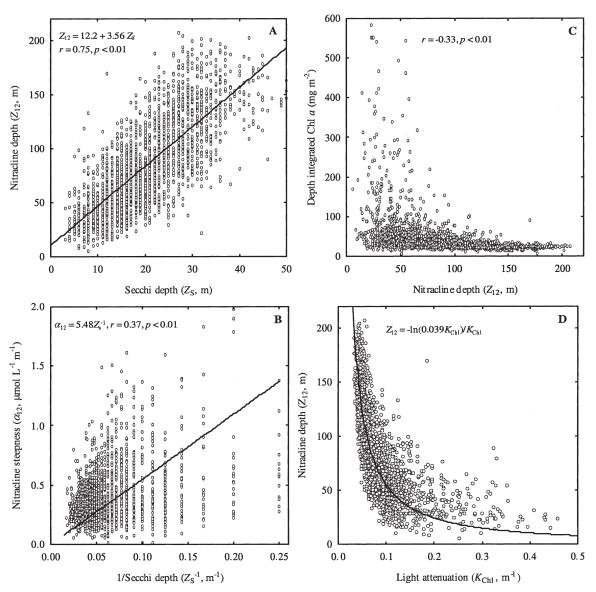
Fig. 2. (A) All pairs (O = 2,187) of observed nitracline depth and Secchi depth and (B) all pairs of observed nitracline steepness and reciprocal Secchi depth. (C) Vertically integrated Chl a versus nitracline depth. (D) Nitracline depth versus the chlorophyll component of the light-attenuation coefficient ( $K_{Chl}$ ) that was calculated according to Eq. 7.
