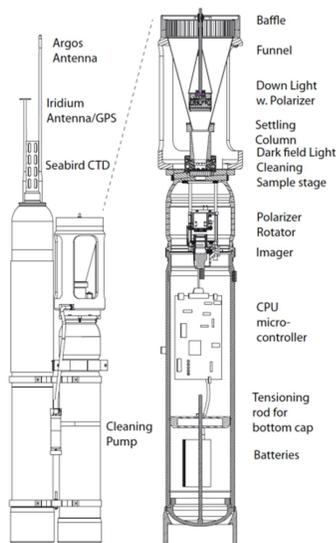
**Fig. 25:** Float and OSR setup for CFE001.
