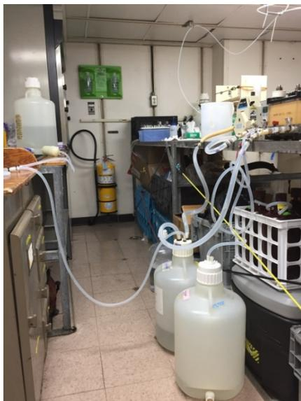
**Fig. 18:** Serial filtration system used to obtain virus-free seawater.
